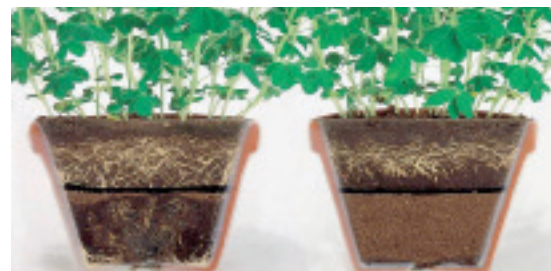
PHOTO: Bituminous Waterproofing without and with antiroot additive Preventol B2.
